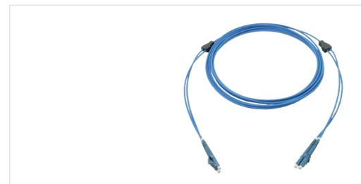
Armoured patch cords are used in customer premises, central offices and in indoor harsh environments. The patch cords provide flexible interconnection to active equipment, passive optical devices and cross-connects. Armoured patch cords are constructed with an helical stainless steel tape over a buffered fibre surrounded by a layer of aramid and stainless steel mesh with an outer jacket.
